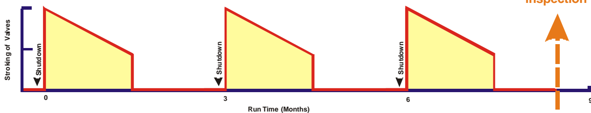
Operation Without Scale-X MFC's (Valves stroked twice daily)
